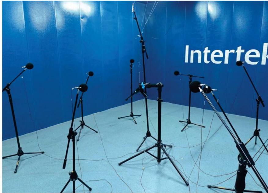
ISO 3744 Figure C.7: Microphone locations
