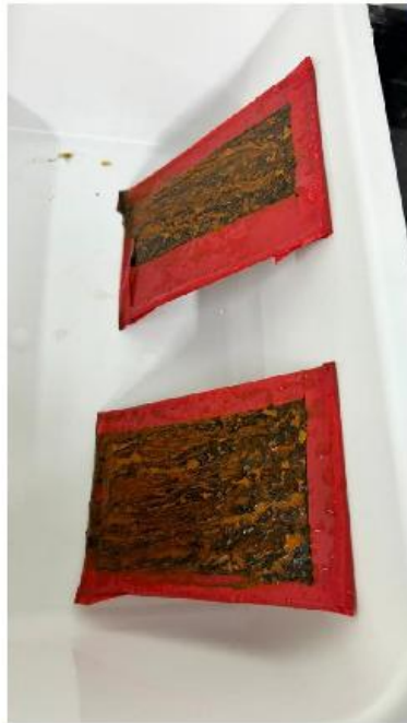
Metallic coated sheets removed from the salt spray chamber
