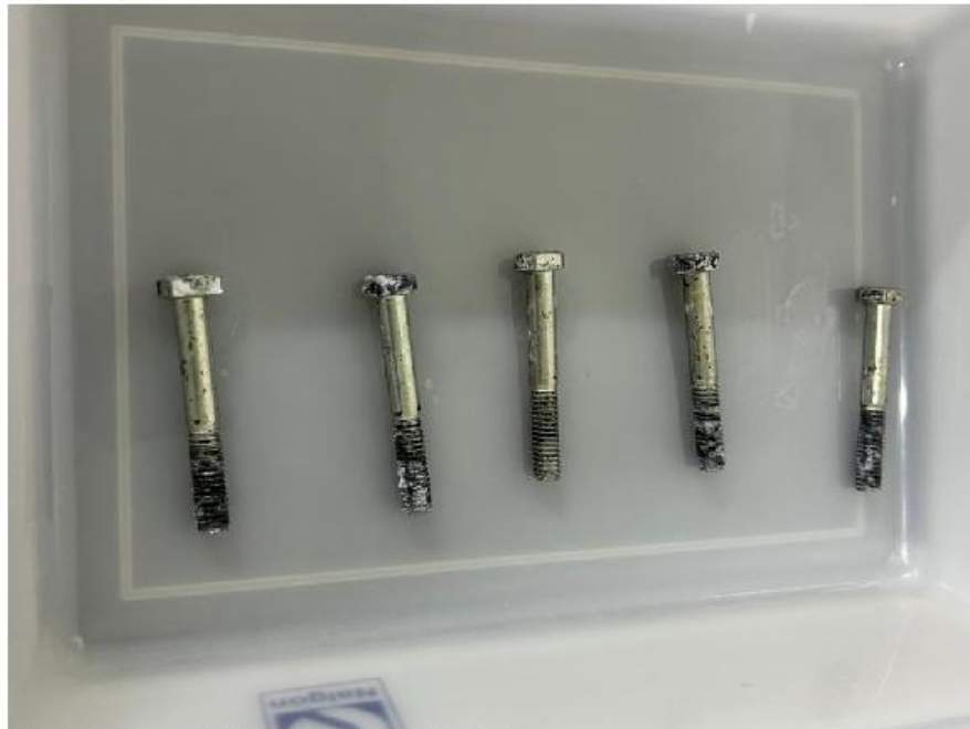
Steel bolts after removal from the salt spray chamber
