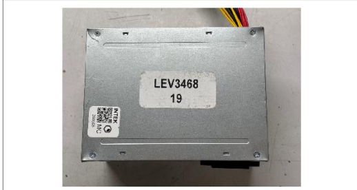
33 - Visual inspection: After vibration – Sample No. 260808
