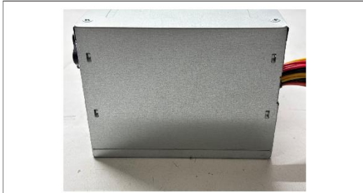
37 - Visual inspection: After vibration – Sample No. 260808
