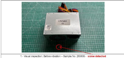
1 - Visual inspection: Before vibration – Sample No. 260806 - screw detached
