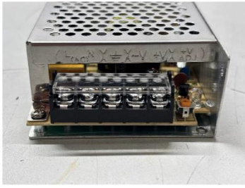
41 - Visual inspection: After vibration – Sample No. 260809
