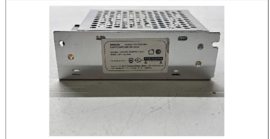
40 - Visual inspection: After vibration – Sample No. 260808
