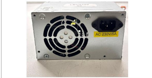
34 - Visual inspection: After vibration – Sample No. 260808
