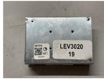
44 - Visual inspection: After vibration – Sample No. 260809
