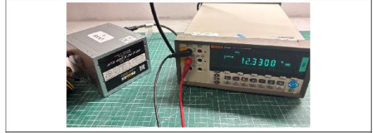
3 - Voltage measurement: Before vibration – Sample No. 260808
